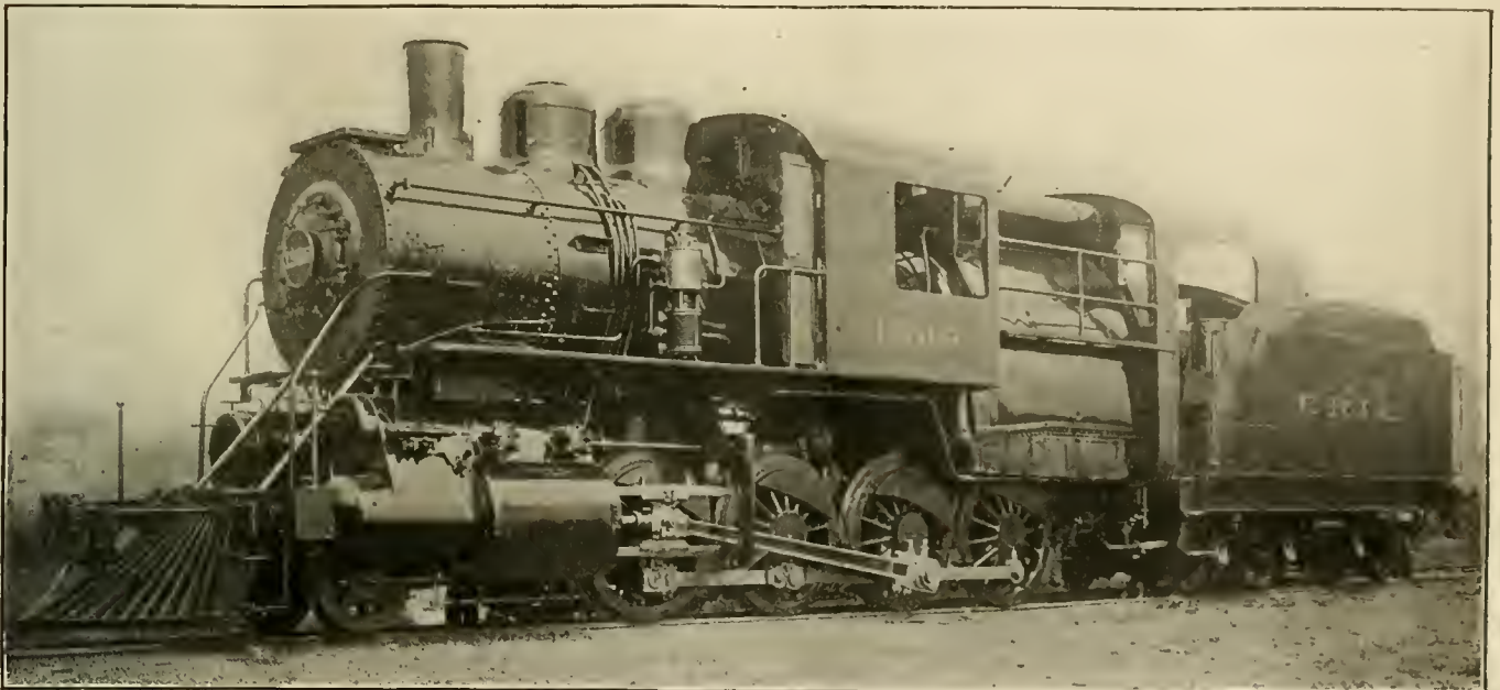
TANDEM COMPOUND CONSOLIDATION—ERIE RAILROAD.
